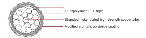
Conductor: Stranded nickel-plated high-strength copper alloy conductor
