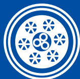
ICEA S-85-625 (原RUS (REA) PE-38)Fig 8 实心PE绝缘&LAP护套电话电缆
