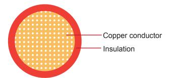
Conductor: Tin coated annealed stranded copper
