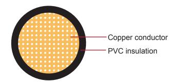
Conductor: Stranded ,bare copper
