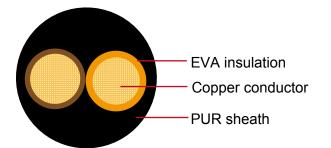
Conductor: Cu-ETP1 tinned according to DIN EN 13602
