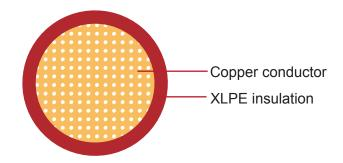
**Conductor:** Annealed stranded copper(Type A)
