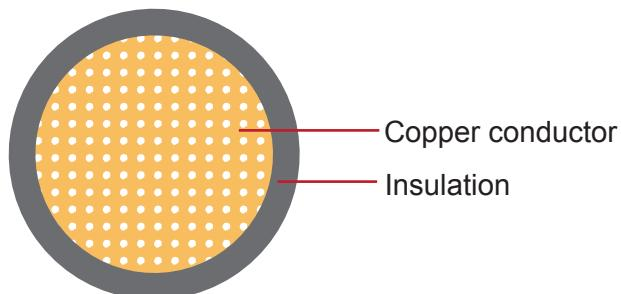
**Conductor:** Annealed stranded copper
