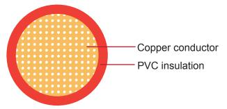
Conductor:Soft-annealed copper according to ASTM B
