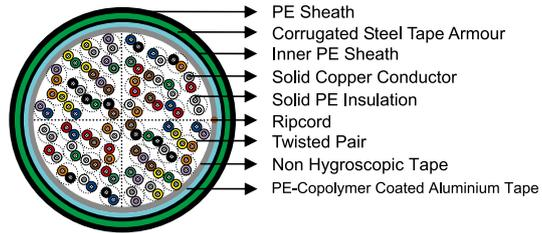
ethylene sheath. An outer polyethylene sheath is applied over the armour.
