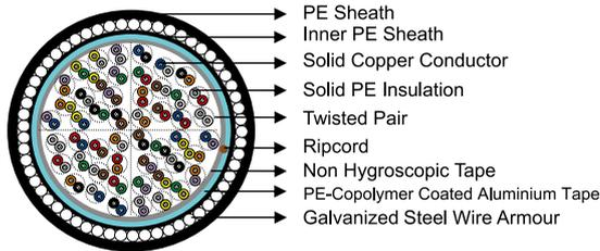
Solid PE Insulated, Steel Wire Armoured & LAP Sheathed (Alpeth) Air Core Cable to ICEA S-85-625
