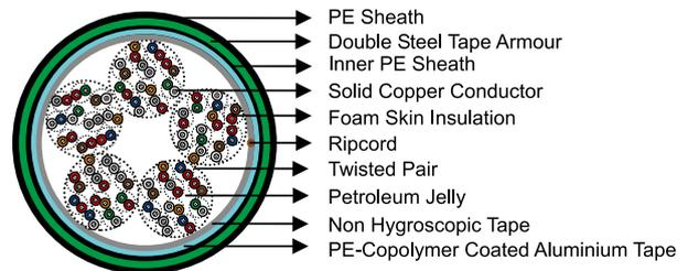
Foam Skin Insulated, Double Steel Tape Armoured & LAP Sheathed Jelly Filled Cable to IEC 60708
