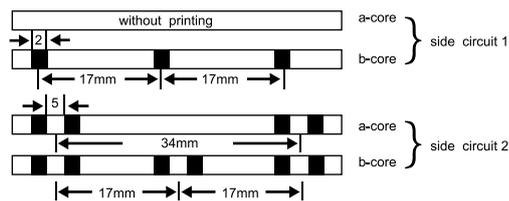
The cores of 5 star quads of a sub unit are counted according to the sequence of basic colours:
