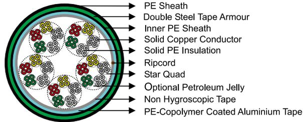
and sheath within the cable core.
