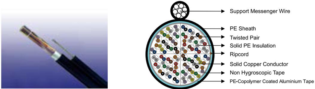
Fig 8 Solid PE Insulated & LAP Sheathed (Alpeth) Air Core Cable to GR-421
