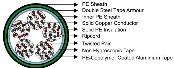
Solid PE Insulated, Double Steel Tape Armoured & LAP Sheathed Air Core Cable to IEC 60708
