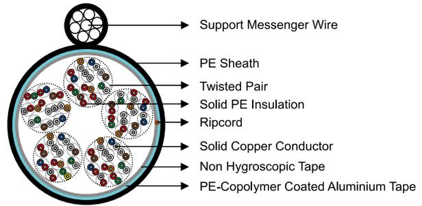
sheath covers both core and support wire in a figure-8 construction.
