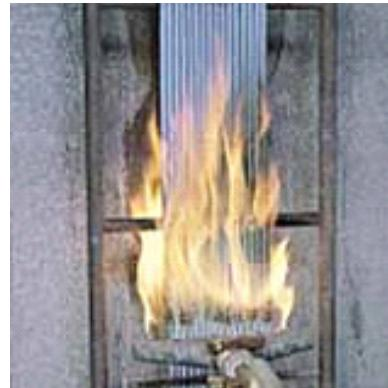
EN 50266-2-3:2001 / BS EN 50266-2-3:2001 / DIN EN 50266-2-3:2001 / VDE 0482-266-2-3:2001-09 / CEI EN 50266-2-1 – Common test methods for cables under fire conditions. Test for vertical flame spread of vertically mounted bunched wires or cables - Part 2-3: Procedures. Category B (Replaced by EN 60332-3-23:2009)
