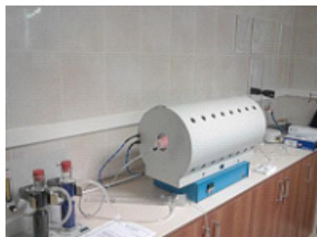
EN 50267-2-3:1999 / BS EN 50267-2-3:1999 / DIN EN 50267-2-3:1999 / VDE 0482-267-2-3:1999-04 / CEI EN 50267-2-3:1999 (CEI 20-37/2-3). Common test methods for cables under fire conditions- Test on gases evolved during combustion of materials from cables- Part 2-3:Procedures. Determination of degree of acidity of gases for cables by determination of the weighted average of pH and conductivity.
