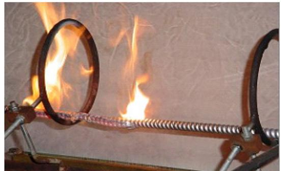
The fire resistant cables are categorized by a letter symbol (e.g. A) or series of symbols (e.g. CWZ) according to the requirements for fire resistance characteristics which they meet, the test temperature selected and the duration of the test for resistance to fire alone in according to BS 6387 as below:
