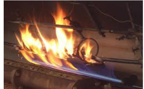
IEC 60331-11 ed1.01 Consol. with am1 (2009-07) – Part 11: Apparatus – Fire alone at a flame temperature of at least 750°C.
