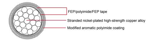
Conductor: Stranded nickel-plated high-strength copper alloy conductor
