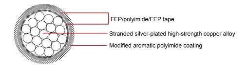
Conductor: Stranded silver-plated high-strength copper alloy conductor
