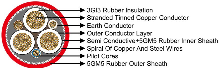
**Conductors:** Flexible stranded tinned copper conductor.
