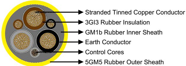
**Conductors:** Flexible stranded tinned copper conductor, class 5 according to DIN VDE 0295.
