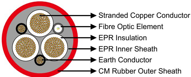
**Conductors:** Flexible stranded copper conductor, class 5 according to DIN VDE 0295.
