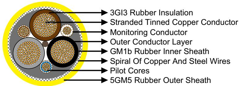
**Conductors:** Flexible stranded tinned copper conductor.
