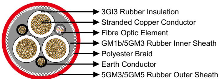
**Conductors:** Flexible stranded copper conductor, class 5 according to DIN VDE 0295.
