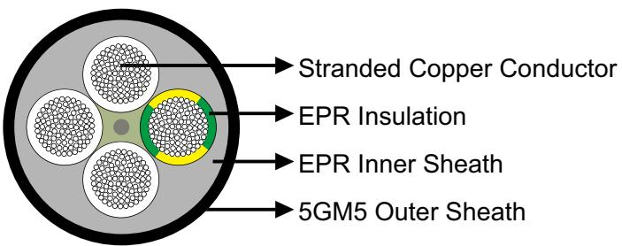
**Conductors:** Flexible stranded copper conductor, class 5 according to DIN VDE 0295/IEC 60228.
