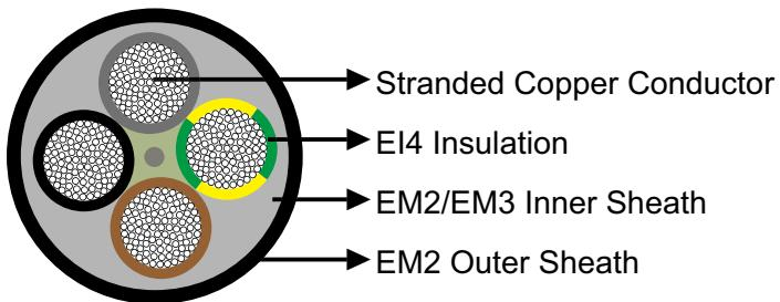
**Conductors:** Stranded copper conductor, class 5 according to DIN VDE 0295/IEC 60228.
