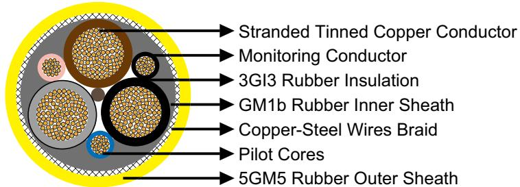
**Conductors:** Flexible stranded tinned copper conductor.
