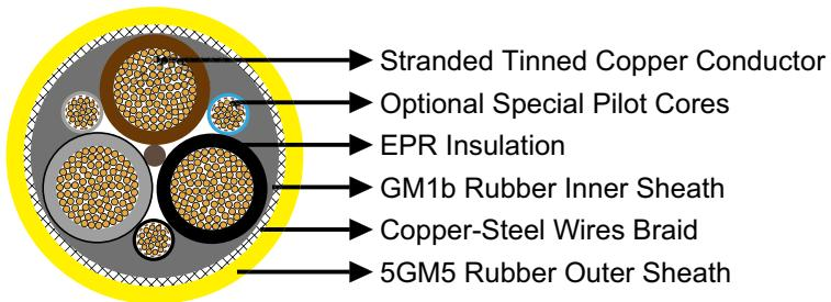
**Conductors:** Flexible stranded tinned copper conductor, class 6 according to DIN VDE 0295.
