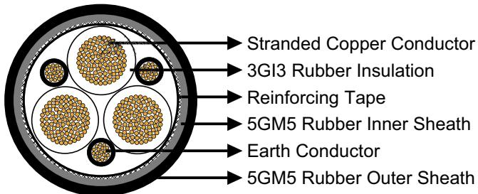
**Conductors:** Flexible stranded tinned copper conductor, class 5 according to DIN VDE 0295.
