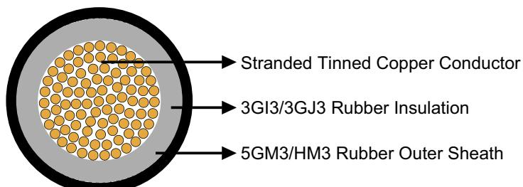
**Conductors:** Stranded tinned copper conductor, class 5 according to DIN VDE 0295/IEC 60228.
