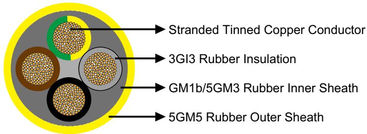
**Conductors:** Flexible stranded tinned copper conductor, class 5 according to DIN VDE 0295.
