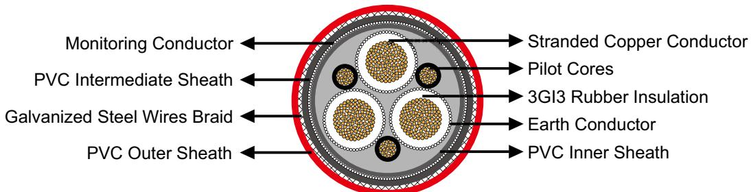
**Conductors:** Flexible stranded copper conductor, class 5 according to DIN VDE 0295.
