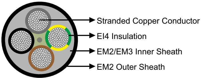
**Conductors:** Stranded copper conductor, class 5 according to DIN VDE 0295/HD 383 S2.
