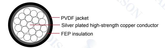
Conductor: Silver plated high-strength copper alloy
