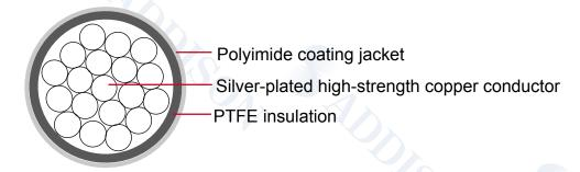
Conductor: Silver-plated high-strength copper alloy
