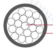
Silver plated high strength copper conductor Fluoropolymer/polyimide tapes
