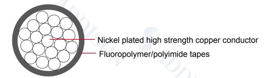
Conductor: Nickel plated high strength copper alloy
