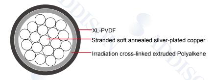
**Conductor:** Stranded soft annealed silver-plated copper conductor **Insulation:** Irradiation cross-linked extruded Polyalkene insulation
