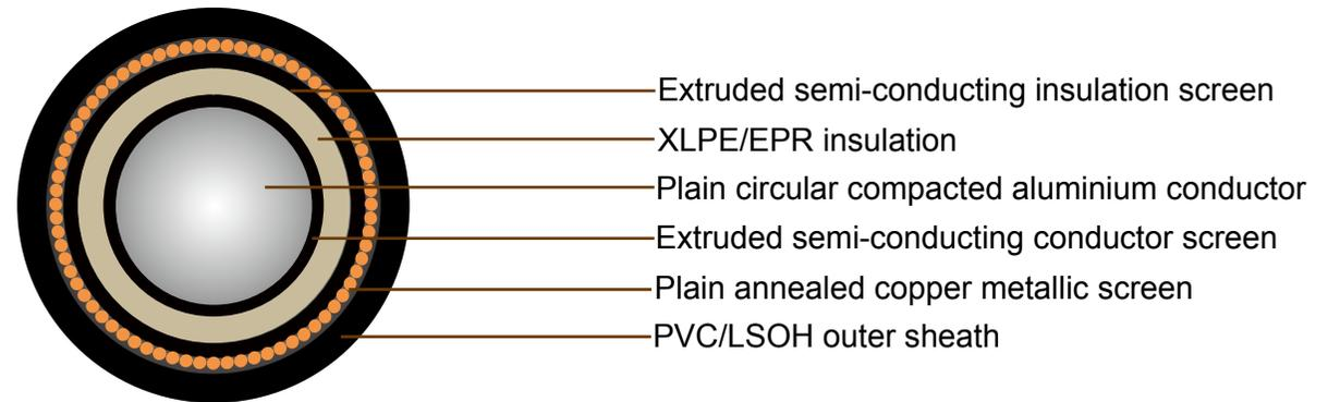
**CONDUCTOR:** Plain circular compacted aluminium to AS/NZS1125
