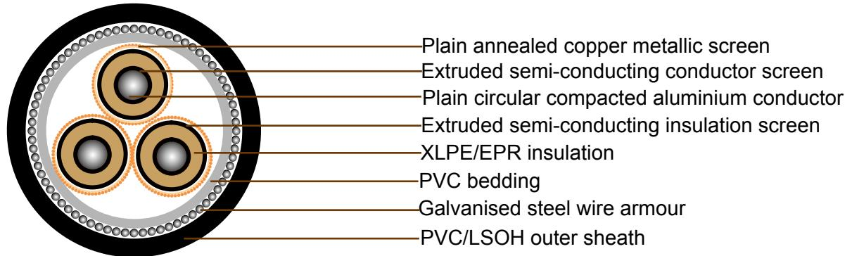
**CONDUCTOR:** Plain circular compacted aluminium to AS/NZS1125
