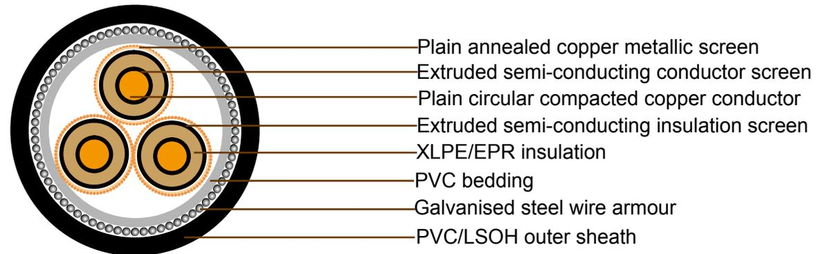
**CONDUCTOR:** Plain circular compacted copper to AS/NZS1125
